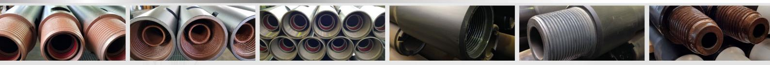
Reverse Circulation Drilling (RC) is a method of drilling which uses dual wall drill pipes that consist of an outer drill pipe with an inner tube. These hollow inner tubes allow the drill cuttings to be transported back to the surface in a continuous, steady flow. Unlike diamond drilling, it compiles sample rock cuttings instead of rock core.
