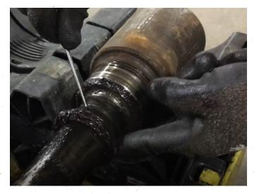
Remove Front Bearing Spacer, clean, and set aside.
