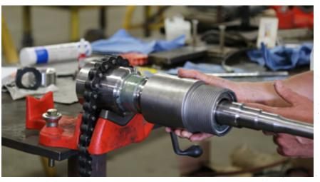
Install Bearing Spacer Ring. It will fit snugly up against last Radial Bearing.
