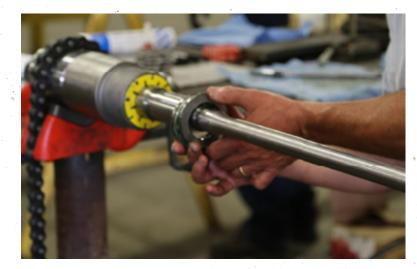
Install Shaft Collar and torque bolts to 25 ft-lbs.
