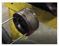
Once Static Piston is free, remove machine screws (set aside and save for later), remove and discard internal seals, and remove and discard external o-rings. Thoroughly clean Static Piston and set aside.
