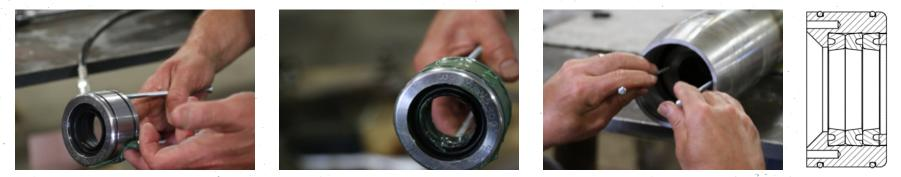
**Lower Housing:** Assemble Lower Housing Assembly. Refer to Assembly page 5. Install three Wiper Rings in Lower Housing with seal facing toward front of housing. (Refer to graphic on Assembly page 5). Install seven (7), pre-packed with grease, radial bearings inside housing.
