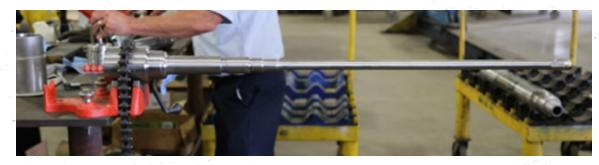
Install Front Bearing Spacer. Internal radius on spacer should face front of Mandrel and fit snugly just behind Front Seal Sleeve. Apply grease to each sleeve on Bearing Mandrel.
