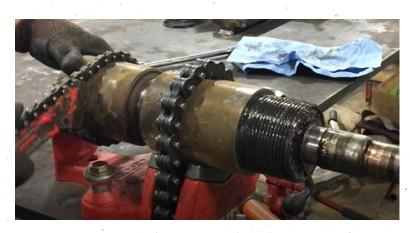
Remove and discard 3 Wiper Seals from Lower Housing. Leave Spiral Retaining Ring in Lower Housing. Do not remove. Thoroughly clean and remove all grease from Lower Housing, including external threads. Set Housing aside.
