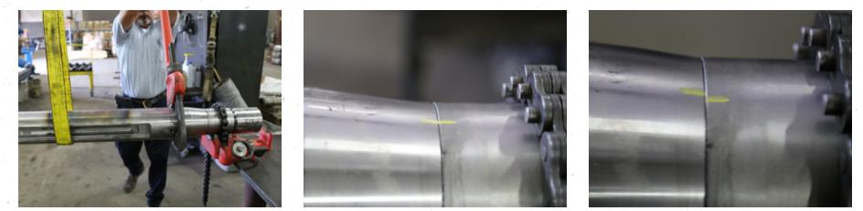
Install Grease Fitting in fill port, pump grease into Fitting until grease comes out Exit point.
