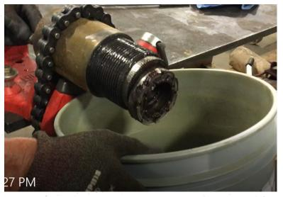
Remove Bearing Mandrel from Lower Housing. Use chain wrench to pull Mandrel forward (can also tap on end of shaft).
