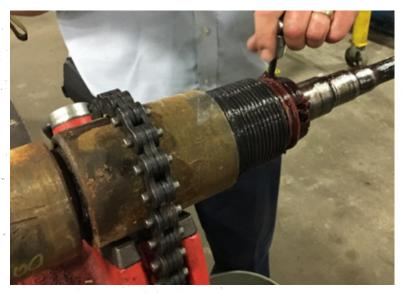
Using punch or screwdriver, remove and discard 7 Radial Bearings from Lower Housing.
