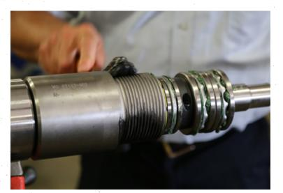
Apply light coat of copper thread compound to external threads of Lower Housing. Do NOT apply grease to box threads in Outer Bearing Housing.
