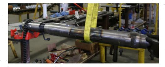
Carefully reposition assembly in chain vise with vise around Lower Housing. Thread Lower Housing onto Outer Bearing Housing. NOTE: **left-hand threads.**
