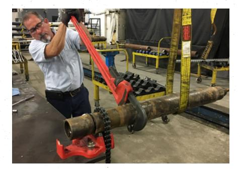
Once broken free, it takes 11-12 revolutions to separate the two pieces. Set OBH aside. NOTE: OBH weighs 115 lbs. Use caution when removing.
