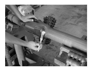
Add new cutter by slipping the journal of the cutter over the spindle and turning clockwise. Insert cutter adapter until flush with the journal face and using the wrench tighten the cutter to the designated torque. Insert retaining bolt and turn counter clockwise (This is a left hand thread bolt). Tighten this bolt to the designated torque
