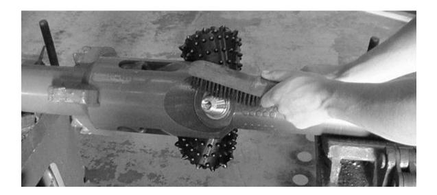
After you are satisfied that all the spindles are in good condition new cutters can be reattached to the hole opener.
