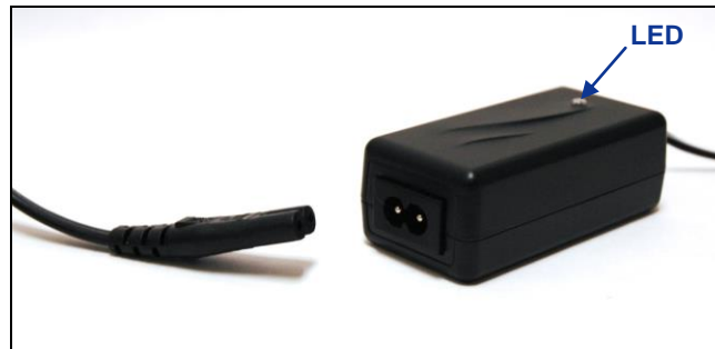
Plug AC Power Cord into Power Unit
