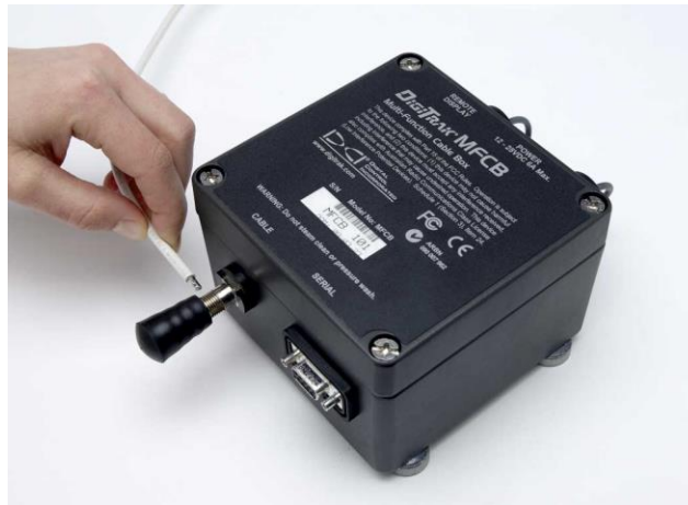
Connecting Transmitter Cable to Cable Box
